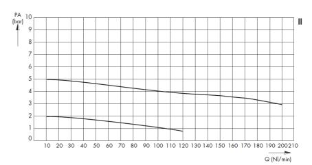
PA = Output pressure PE = Input pressure Q = Flowing through I Inlet pressure sensivity
