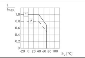
Fig. 20: Permissible current load
