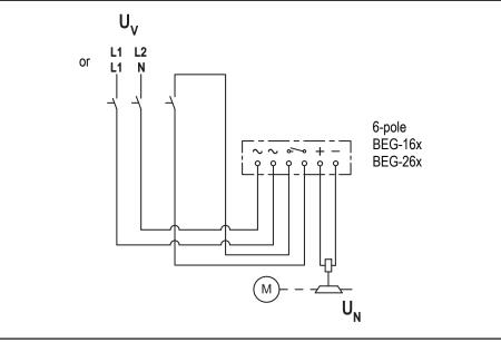
Fig. 17: Supply: Phase-phase or phase-N via 6-pole rectifier
