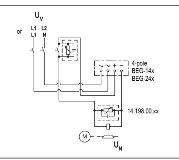
Fig. 18: Supply: Phase-phase or phase-N via 4-pole rectifier
