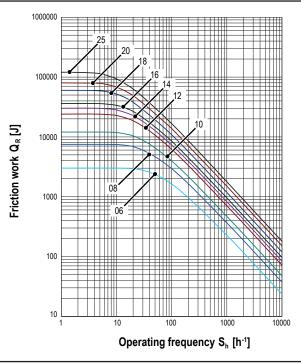
Fig. 5: Friction work as a function of the operating frequency
