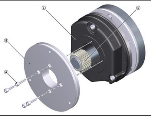
Fig. 18: Installing the intermediate flange
