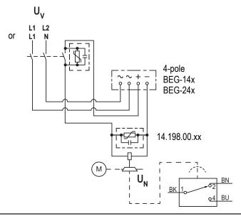
Fig. 29: Supply: Phase-phase or phase-N via 4-pole rectifier
