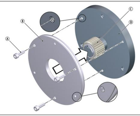
Fig. 15: Flange mounting for sizes 06 - 16
