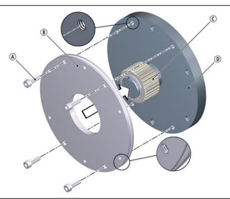
Fig. 16: Flange mounting for sizes 18 – 20
