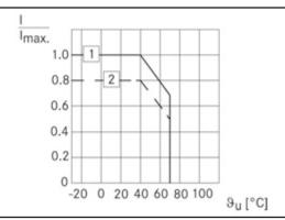
Fig. 31: Permissible current load
