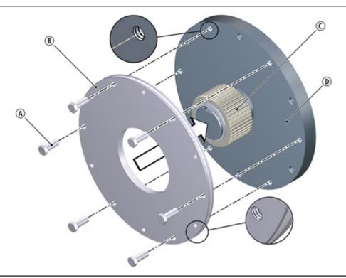
Fig. 17: Flange mounting for size 25
