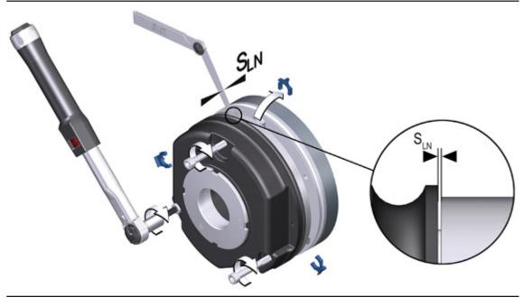
Fig. 12: Tightening the screws with a torque wrench
