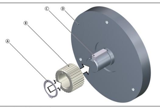
Fig. 9: Installing the hub onto the shaft
