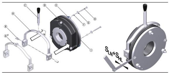
Fig. 21: Assembly of the hand-release BFK458
