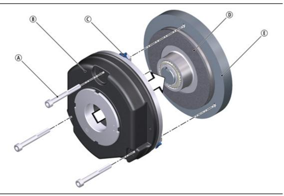
Fig. 11: Mounting the complete stator
