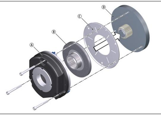
Fig. 14: Mounting the friction plate
