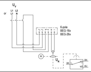
Fig. 28: Supply: Phase-phase or phase-N via 6-pole rectifier
