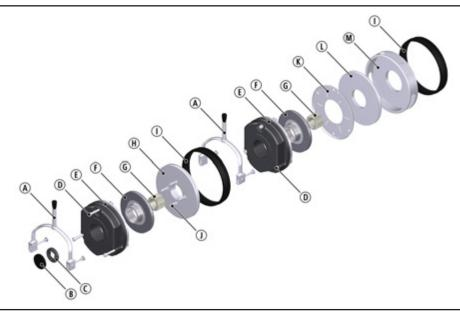
Fig. 35: INTORQ double spring-applied brake BFK458-06 to 25
