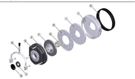
Fig. 40: INTORQ spring-applied brake BFK458-06 to 25
