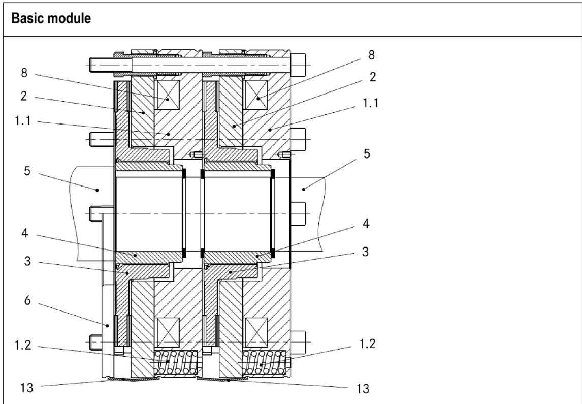
**Fig. 1 Design of a BFK455 spring-applied brake**
