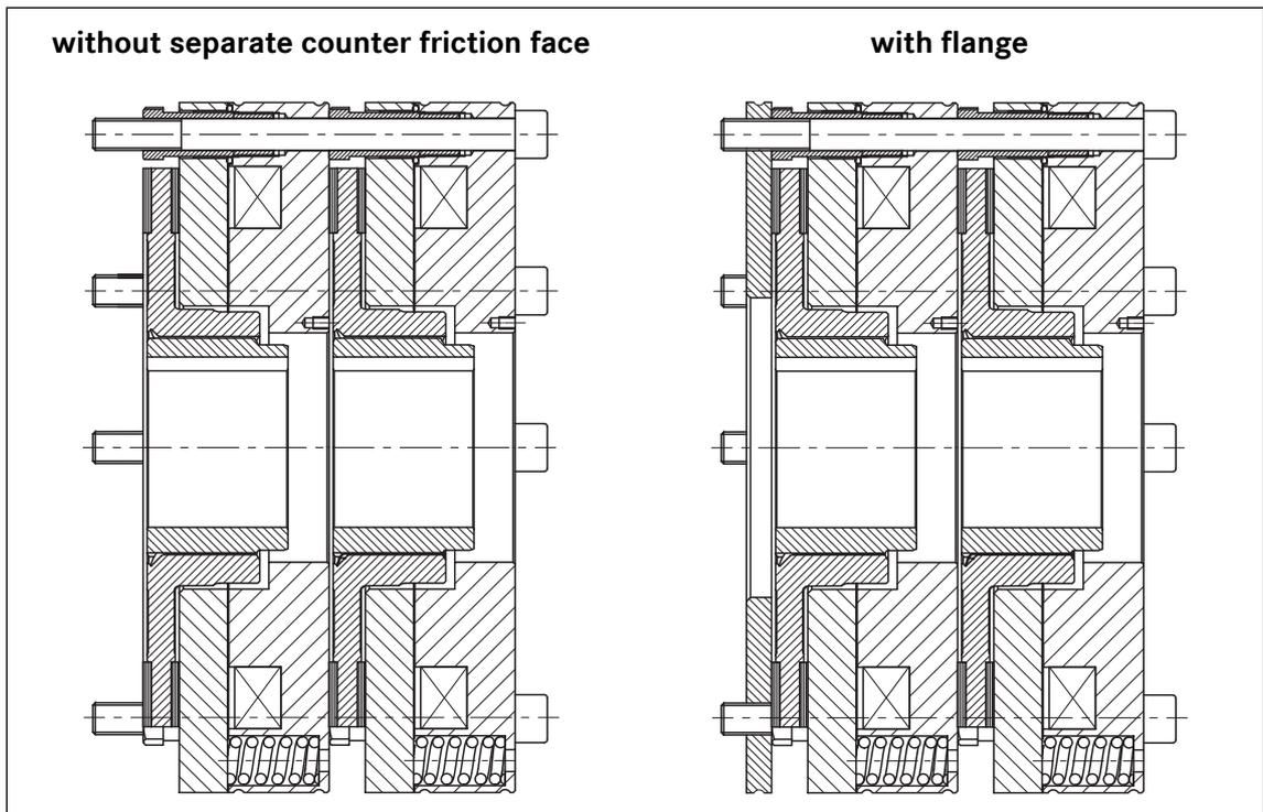
**Assembly of the counter friction faces**
