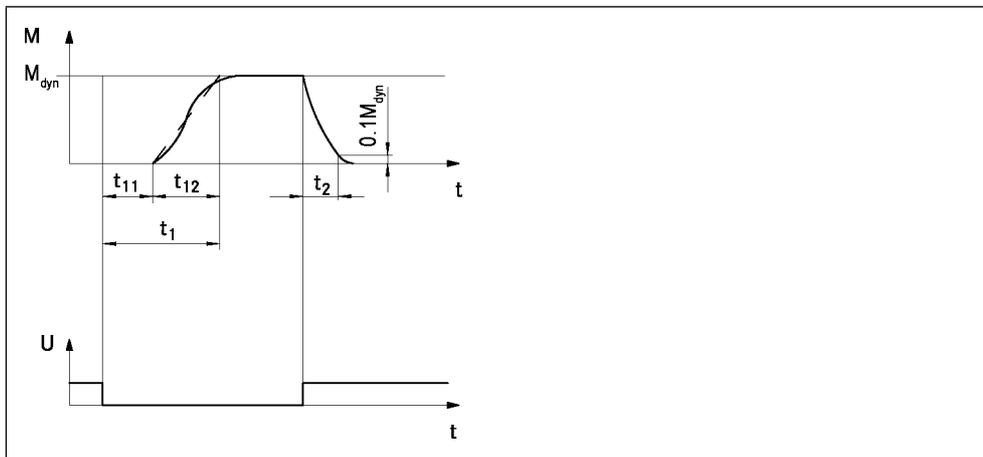
Fig. 2 Operating/switching times of the spring-applied brakes
