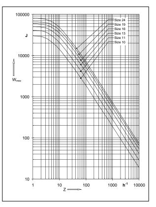
Fig. 30/2: Max. switching work  $W_{max}$  <sup>6)</sup> per switching operation as a function of the number of switching operations per hour Z (built-in brakes; values based on n=1500 rpm)
