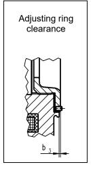
Table 19/1: Change in the M<sub>4</sub> transmissible torque from 1 mm axial adjustment of the adjusting ring (7); adjusting ring clearance b<sub>3</sub> limit values
