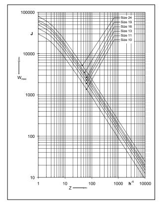
Fig. 30/1: Max. switching work  $W_{max}$  <sup>6)</sup> per switching operation as a function of the number of switching operations per hour Z
