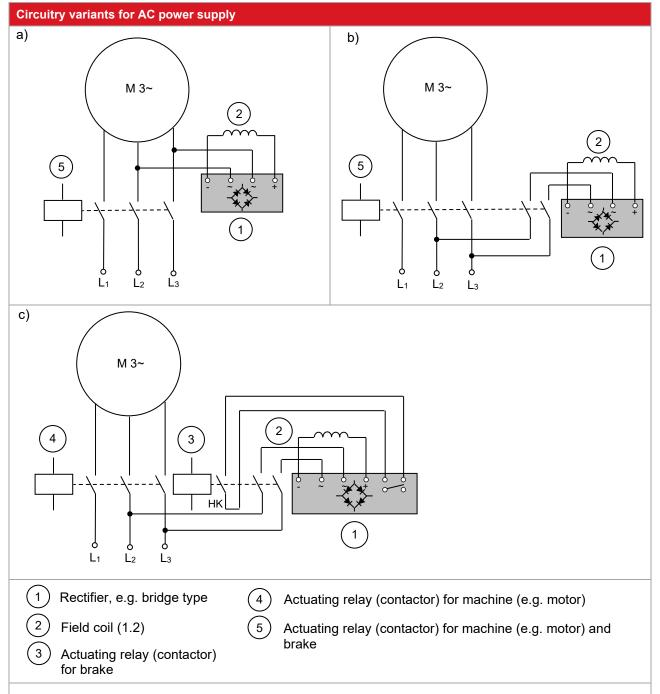
Fig. 26/1: DC side and AC side switching of the spring-applied single-disc brake with connection of the field coil (1.2) to an AC power source via a rectifier (example)
