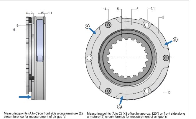
Fig. 15/3: Location of the measuring points (arrow marks) for measuring the air gap 's' of brake type SL 502..A00 (example), shown without hub (7)
