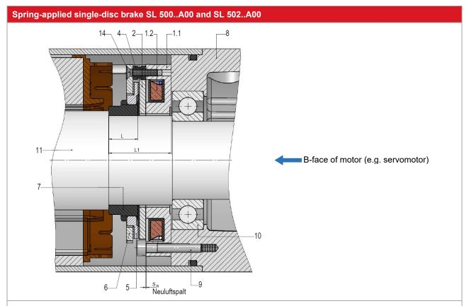
Fig. 14/1: Flange side mounting of spring-applied single-disc brake SL 500..A00 (example) to the motor (e.g. servomotor); contact of hub (7) with stop shoulder of machine shaft (e.g. motor shaft) (11); assembly of hub (7) and machine shaft (e.g. motor shaft) (11) by interference fit (see Section 4.1.2)
