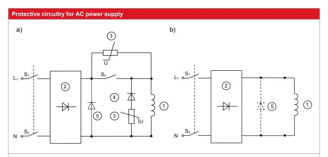
Fig. 27/1: DC side and AC side switching of the spring-applied single-disc brake and connection of the field coil (1.2) via rectifier to a AC power source (circuit examples)
