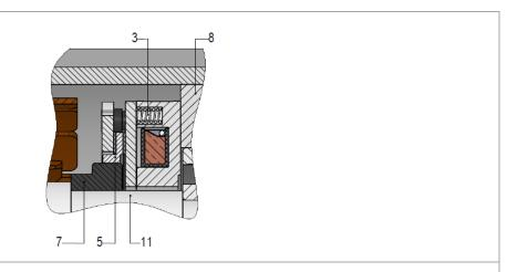
Fig. 15/1: Interference fit assembly of hub (7) and machine shaft (e.g. motor shaft) (11)
