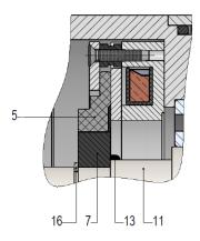
Fig. 15/2: Feather key assembly of hub (7) and machine shaft (e.g. motor shaft) (11)
