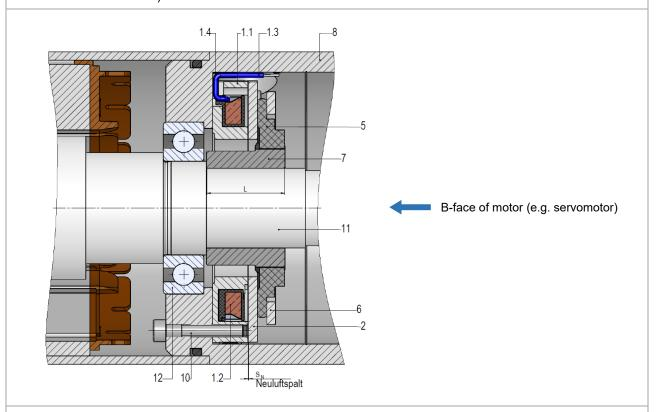
Fig. 14/2: Front side mounting of spring-applied single-disc brake SL 502..A00 (example) to the motor (e.g. servomotor); contact of hub (7) with stop shoulder of machine shaft (e.g. motor shaft) (11); assembly of hub (7) and machine shaft (e.g. motor shaft) (11) by interference fit (see Section 4.1.2)
