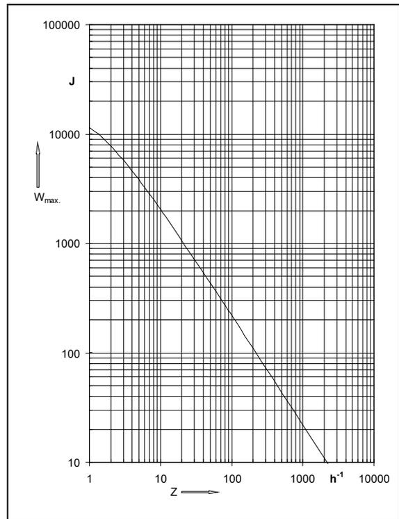
Fig. 24/1: Max. switching work  $W_{max}$  per switching operation as a function of the number of switching operations per hour  $Z$  (values based on  $n=1500$  rpm)
