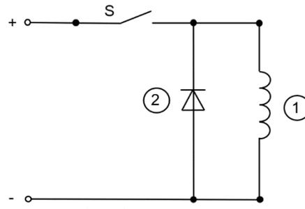
Fig. 24/1: DC side and AC side switching of the spring-applied single-disc brake and direct connection of the field coil (1.2) to a DC power source (circuit examples)
