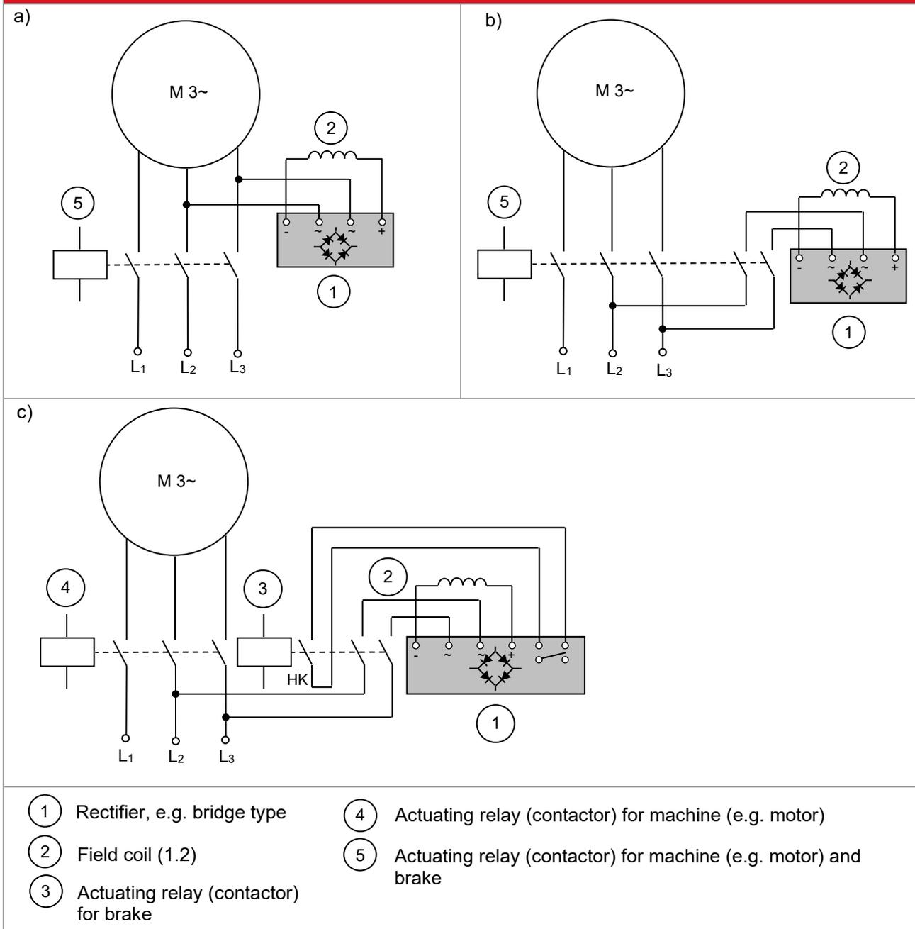
Fig. 26/1: DC side and AC side switching of the spring-applied single-disc brake with connection of the field coil (1.2) to an AC power source via a rectifier (example)
