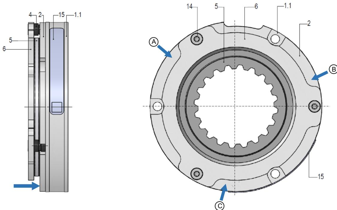
Measuring points (A to C) on front side along armature (2) circumference for measurement of air gap 's'
