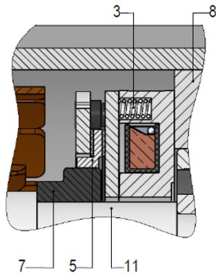
Fig. 15/1: Interference fit assembly of hub (7) and machine shaft (e.g. motor shaft) (11)
