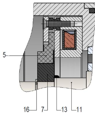
Fig. 15/2: Feather key assembly of hub (7) and machine shaft (e.g. motor shaft) (11)
