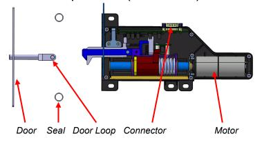
The door is open and can be closed without operators having to exert much force.
