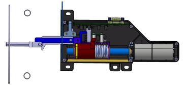
The process (e.g. baking) is finished. The motor drive runs **forward** to open the door to an about 30 mm gap at sensor #5. The heat can escape, and the baking process terminates. To prevent operators from being burnt, the door may stay locked for a customisable time.
