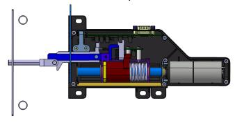
The door latches onto the door loop but need not be closed completely. The door locks preliminarily and prevents the door from opening.
