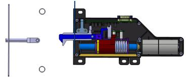
To return the lock to its home position, the motor drive now needs to move **backward** to sensor #1.
