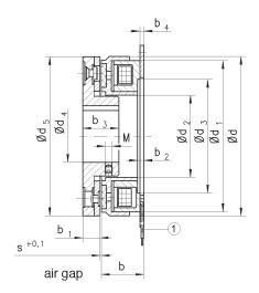
1 flying 2x0.14mm² (size 04) leads 2x0.25mm² (size 06.07) 2x0.50mm² (size 09.11) 2x1.00mm² (size 14)
