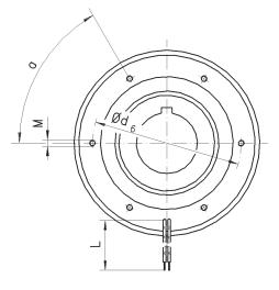
1 flying 2x0.14mm<sup>2</sup> (size 04) leads 2x0.25mm<sup>2</sup> (size 06.07) 2x0.50mm<sup>2</sup> (size 09) 2x1.00mm<sup>2</sup> (size 11.14.17) 2x0.82mm<sup>2</sup> (size 21)
