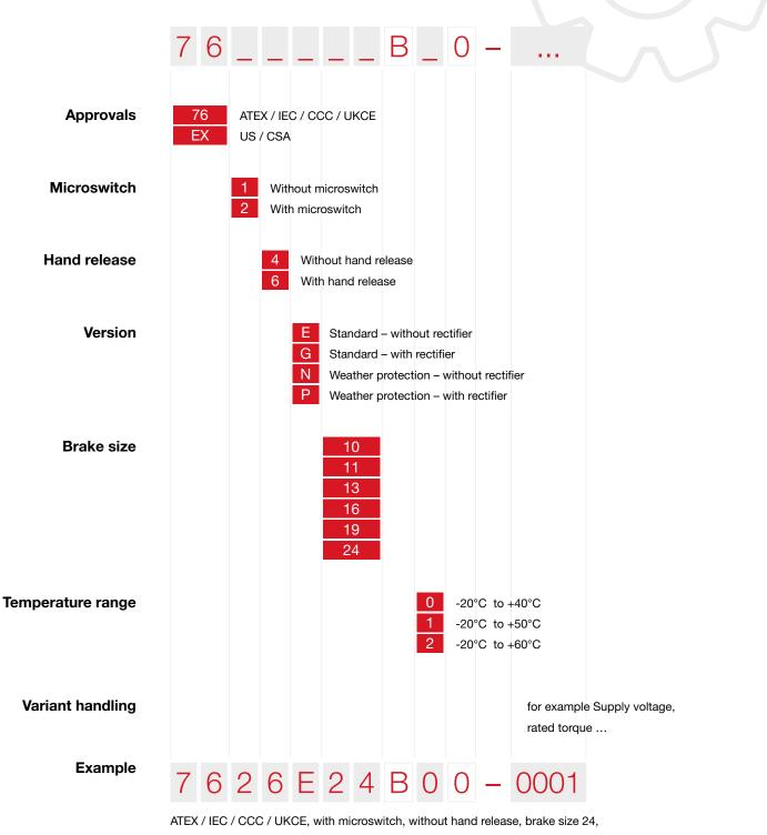
temperature range -20°C to +40°C, 205V DC / 270 Nm
