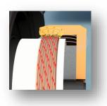
Contrary to the loudspeaker where the magnet is rigidly attached to a basket, with the IPG, the magnet is mounted axially-movable in a soft metal-spring suspension. On the one hand, this achieves a low magnet resonance frequency and a particularly good performance, especially at low frequencies. On the other hand, this results in a high degree of robustness as well as a high protection class.
