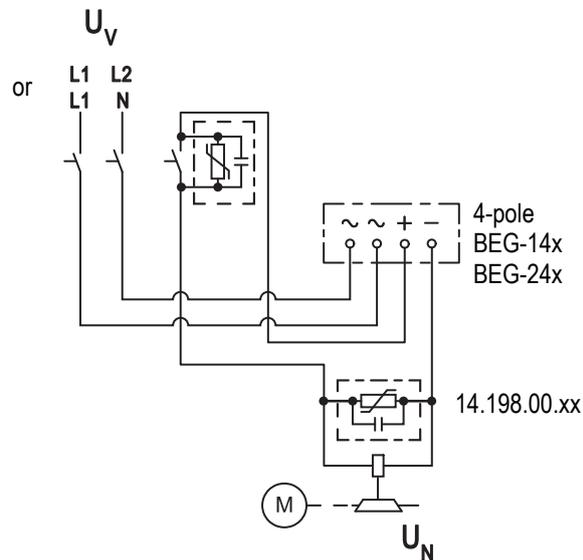
Fig. 18: Supply: Phase-phase or phase-N via 4-pole rectifier
