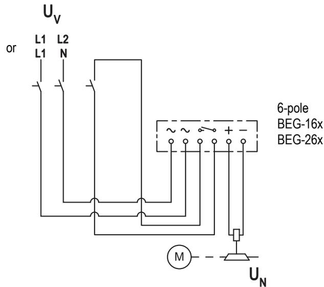
Fig. 17: Supply: Phase-phase or phase-N via 6-pole rectifier
