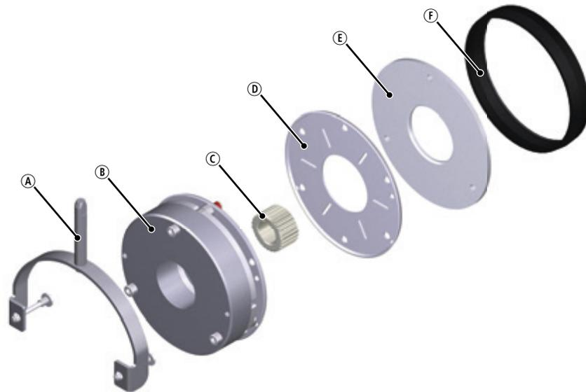
Fig. 21: Spring-applied brake INTORQ BFK557 - sizes 06 to 12
