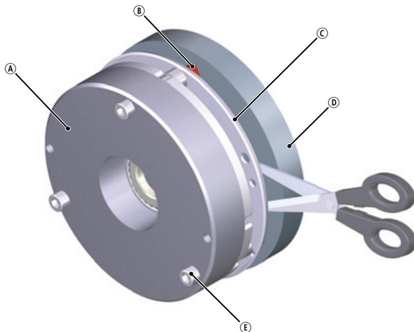
**Fig. 7: Remove the assembly aid**
