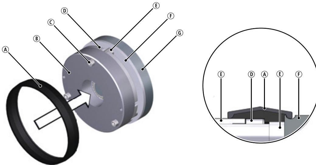
**Fig. 10: Assembly of the cover ring with flange**
