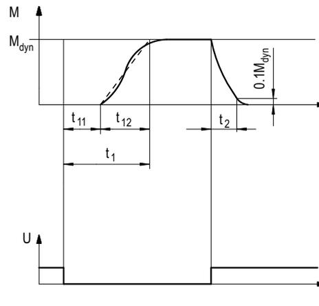
**Fig. 2: Operating/switching times of the spring-applied brakes**
