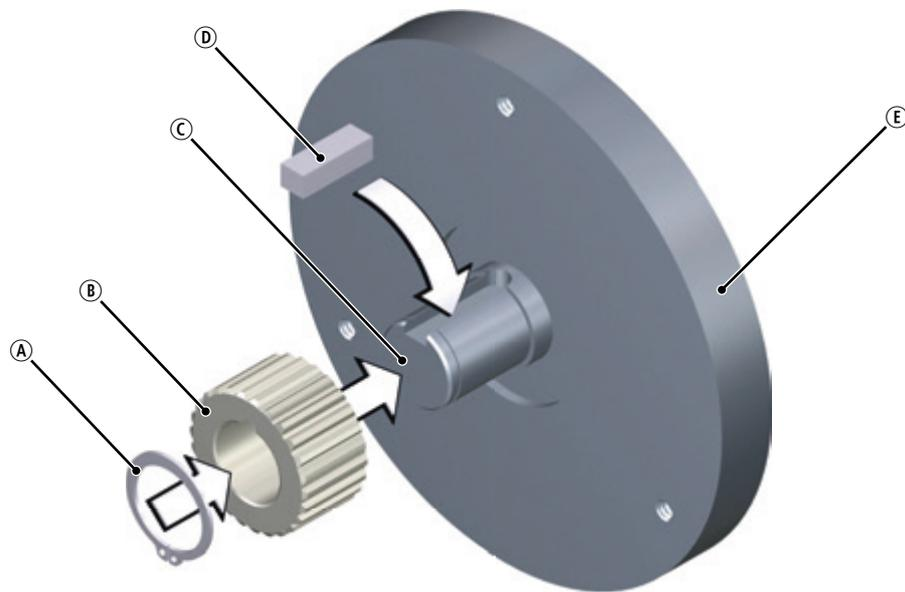
**Fig. 5: Mounting the hub**
