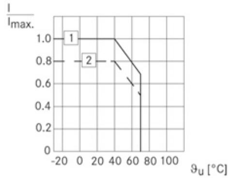
Fig. 20: Permissible current load
