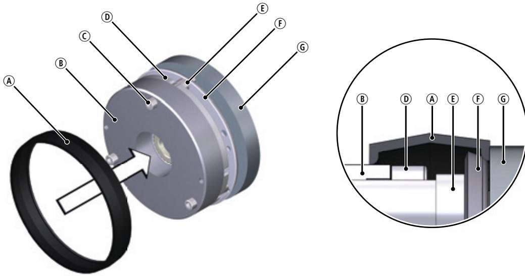
**Fig. 9: Assembly of the cover ring with friction plate**
