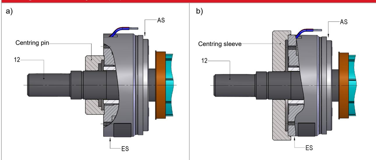
Fig. 23/1: High Torque brake types 86 611..P00 with armature type 800
