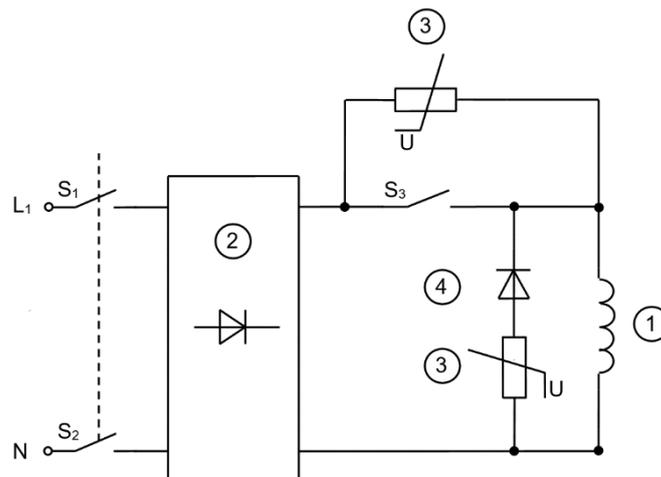
Fig. 30/1: Circuit examples for recommended protective measures for DC side switching of the High Torque brake when the field coil (1.2) is connected to an AC power source via a bridge rectifier without internal protective circuitry elements
