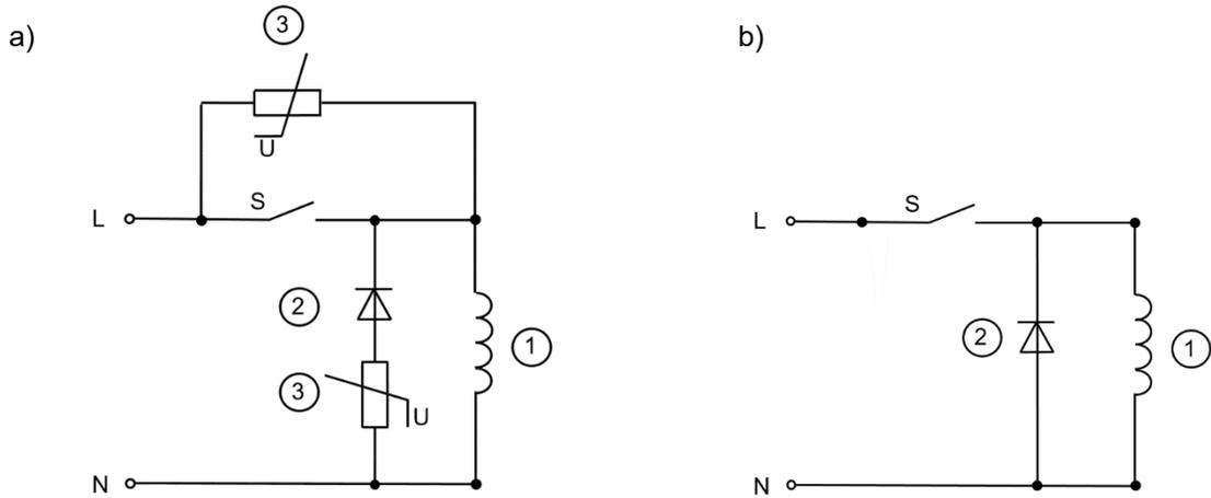
Fig. 28/1: DC side and AC side switching of the High Torque brake with direct connection of the field coil (1.2) to a DC power source (example)
