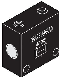
Kuhnke has developed a high-quality range of non-return valves for applications requiring non-return and check functions. The check valve closes by means of a spring when the outlet pressure is greater or the same as the input pressure. A speciality in the range is the shuttle or dual-pressure valve. Using this AND/OR logical functions are possible in a pneumatic control. Our fast vent valve NW 2 ensures fast venting of the cylinder volumes.
